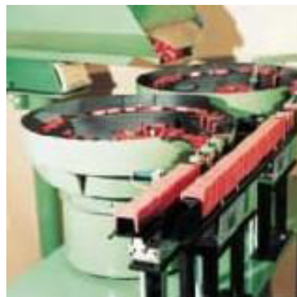
Stored brackets for yarn bobbins are oriented with this feeding device and fed to two lanes of a winding machine
