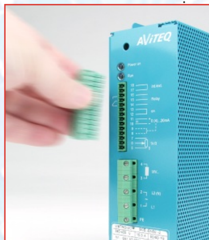
Standard: Pluggable signal-terminal-strip
